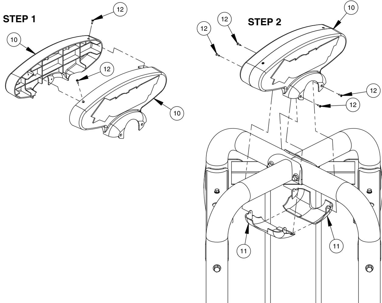
NOTE: THIS STEP CAN ALSO BE COMPLETED WITH THE TOP CAP FROM STEP 1 PLACED AT 90 DEG. TO THE POSITION SHOWN.
